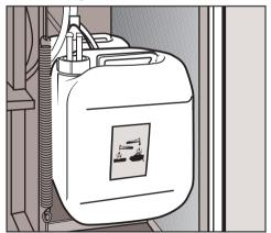
■ Take the storage container out of the unit, open it and fill with the agent required. Observe the color code.
